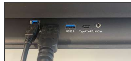
Front Ports with USB Type-B and HDMI cable connected.
