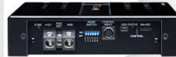
Control Processor ( its Controls Power On/Off, AV Receiver Control ,Lighting Control, Air Con & Newline Panel Control)
