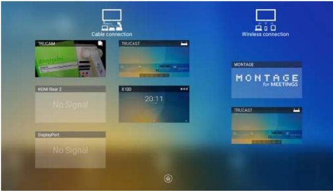
The first time you turn the screen on, only the cable connections appear in **Connection**. Wireless connection can be added in the **Newline Extension** setting. In this case, the name and icon of the HDMI on the left cabled channel change as the Trucast application is enabled or an external product is connected. For details on the configuration, see section “Newline Extension”. After the setting is successful, connect the Trucast, X10D and Trucam to corresponding HDMI ports of the screen.
