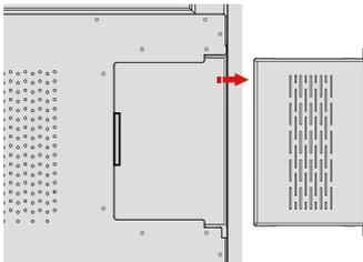
**Step 2:** Push the internal PC into the internal PC port at the rear of the display from right to left.
