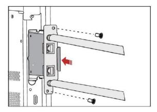
Step 3: Use the new M3\*6 screws provided with the Wi-Fi module to secure it to the panel. Note: Do not over tighten screws.
